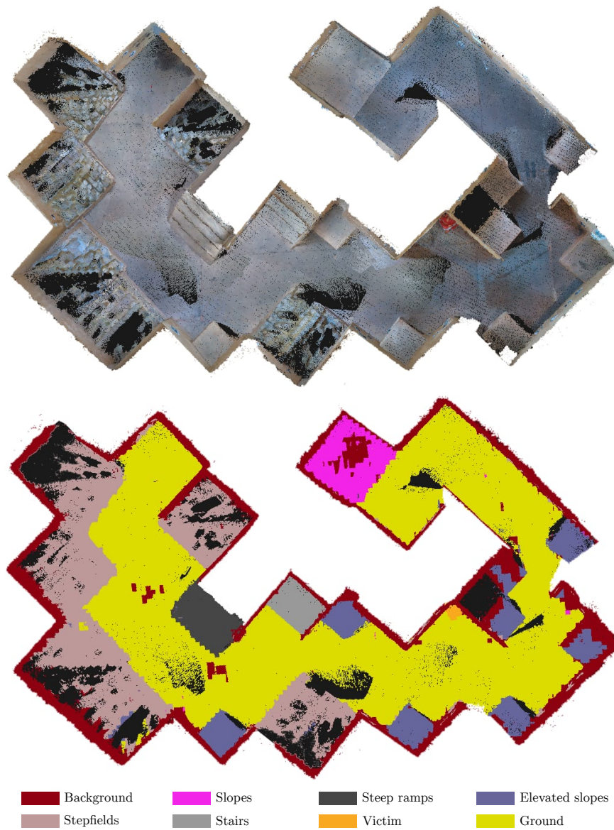
Figure 10.3: Dense semantic map generated by our approach in the RoboCup Rescue League competition field. The upper image shows the colored point-cloud map of the RRL test field (view from the top). The lower image shows the corresponding semantic map, including eight different terrains and objects.
