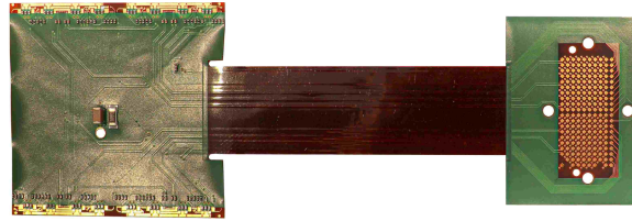
Figure 5.16: Flex PCB used for the RD53A quad chip assembly for the SP prototype.
