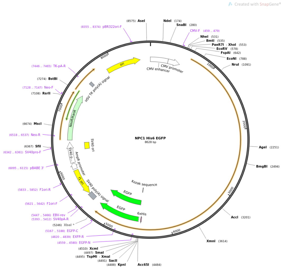
Fig.3.2. Map of the NPC1 His6 EGFP plasmid: Full sequence map of NPC1 His6 EGFP (plasmid #53521). Picture downloaded from addgene website.
