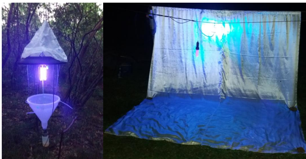
Figure 2.3. Light trap in the field (left). Manual collecting from a white sheet illuminated with UV light in the field (right).
