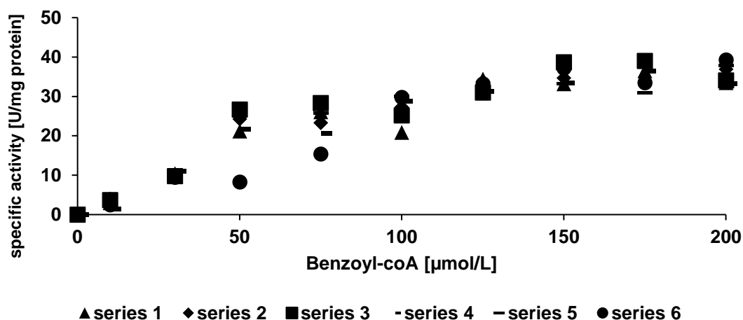
Figure 4.24: Intra-assay variation study of 1.5 µg purified GLYAT wild-type by measuring kinetic curve 6x with the same sample (n=6, technical replicates). Benzoyl-coA concentrations from 0 to 200 µmol/L were applied and specific activities were calculated; v_{max} and K_M values were calculated using Excel Solver tool. Variations coefficient for v_{max} is 8 %, whereas for K_M 19 % were calculated.
