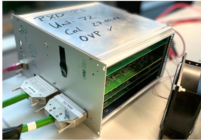
Figure 6.6: Custom-made power supply (LMU-PS) for the Belle II PXD. The side view shows the modular structure with DC/DC and regulator cards. Two 18m-long cables are used to provide the module with power. The Ethernet connection is used for remote control.
