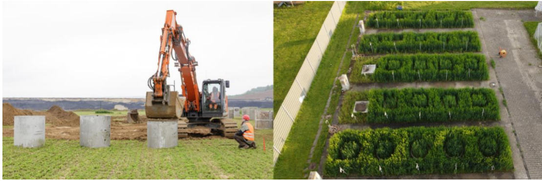
Figure S5.1 Filling of the lysimeters with intact soil (left) and the lysimeter installation on the campus of Forschungszentrum Jülich (right).
