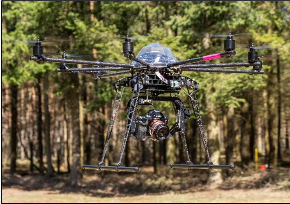
Figure 7: OctoXL 6S12 Octocopter mounted with a fixed lens Sony A7r RGB camera.
