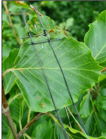
Figure 15: The LAT-B2 (Ecomatik, 2022) leaf temperature sensor which was mounted in the upper tree crown and used for validating the TIR imagery.
