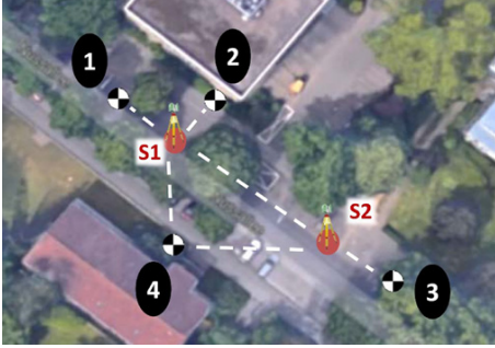
Figure 9: Sketch of the experiment used in 1 st TLS calibration example. Four targets (1–4) measured from two scanner stations (S1 and S2).
