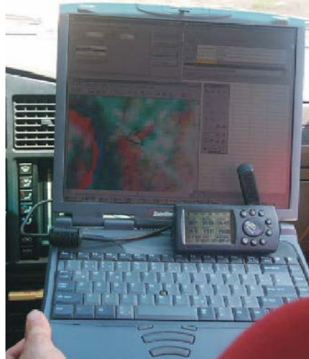
Figure 2.7: Example of the real time GPS link of ERDAS imagine in the field (adapted from Thamm and Schmidt, 2001)
