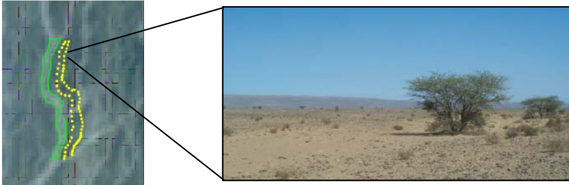
Figure 2.8: Position shift of the ground truth data due to geo-location errors. The yellow points represent the data obtained in the field, the green polygon represents the shifted dataset. Coordinates of the photo (UTM): 809370/3348542
