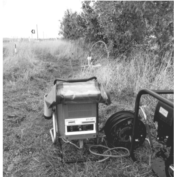
Figure 3.22: View at site BV in western direction over the grass verge. In foreground is the control box of the pump and the generator. In background is the outlet tube for extracted ground water.
