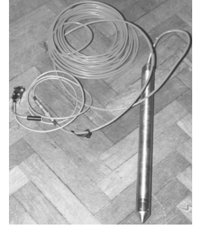
Figure A.7: Pressure Transducer TROLL-4000, used in B1 OE , B2 OE , B3 OE .
