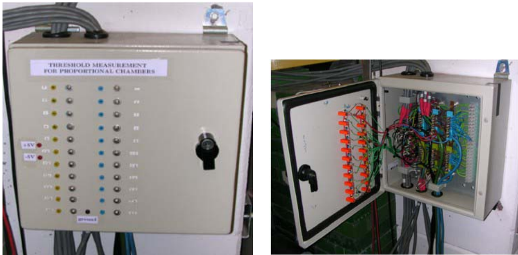
Figure C.1: Distribution box for MWPCs: thresholds and power supply cables ( \pm 5 \text{ V} ) for PCOSIII cards.
