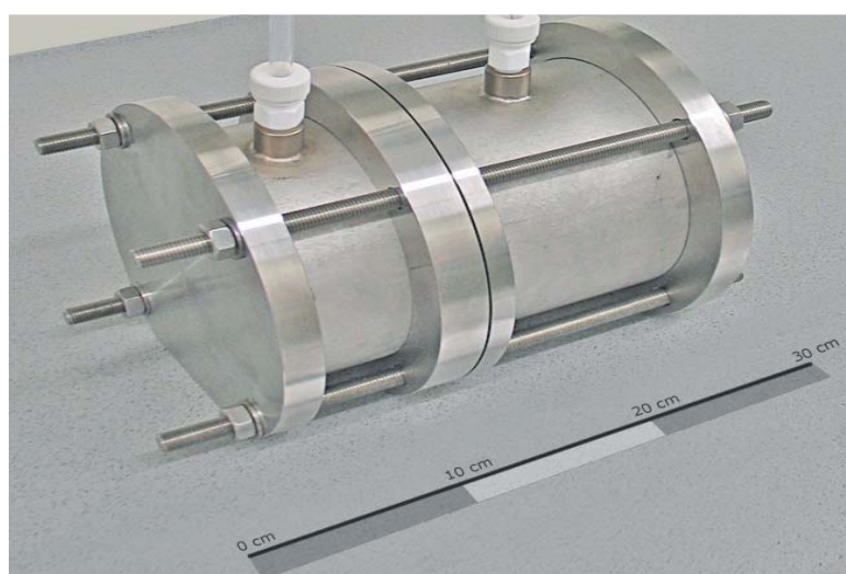
Fig. 6-2: Stainless steel diffusion cell (build up cell).
