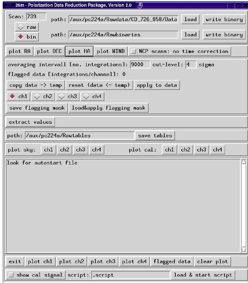
Figure 3.11: The raw data reduction program that reads the raw data and does flagging, processing and gridding. The user can examine the data on different types of displays. Parameters for data flagging can be chosen and individual channels can be searched for interference. Data can be stored on disk in a space saving AIPS++ binary file format.
