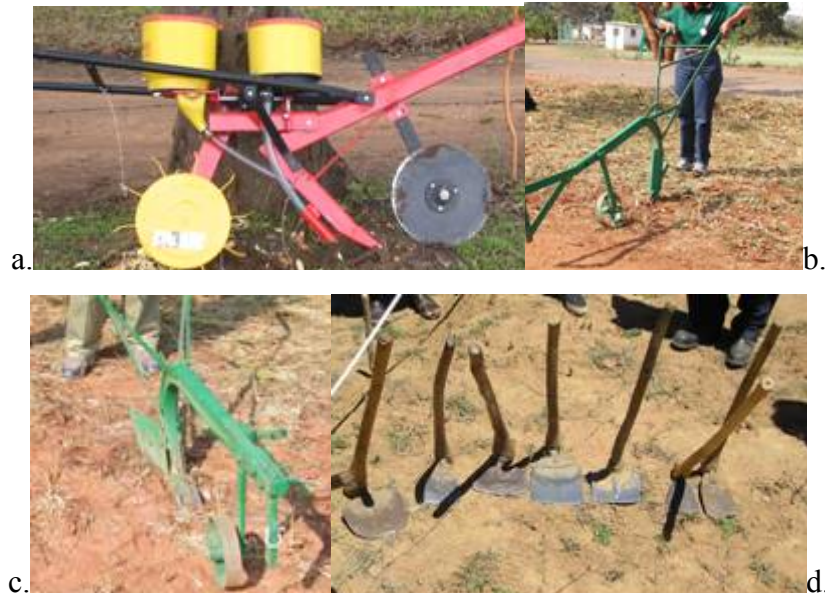
Figure 1.1: Four tillage implement used during the experiments (a) direct seeder (b) ZimPlough ripper manufactured in Zimbabwe (c) Magoye ripper originally designed in Zambia and (d) hand hoes for making basins and weeding
