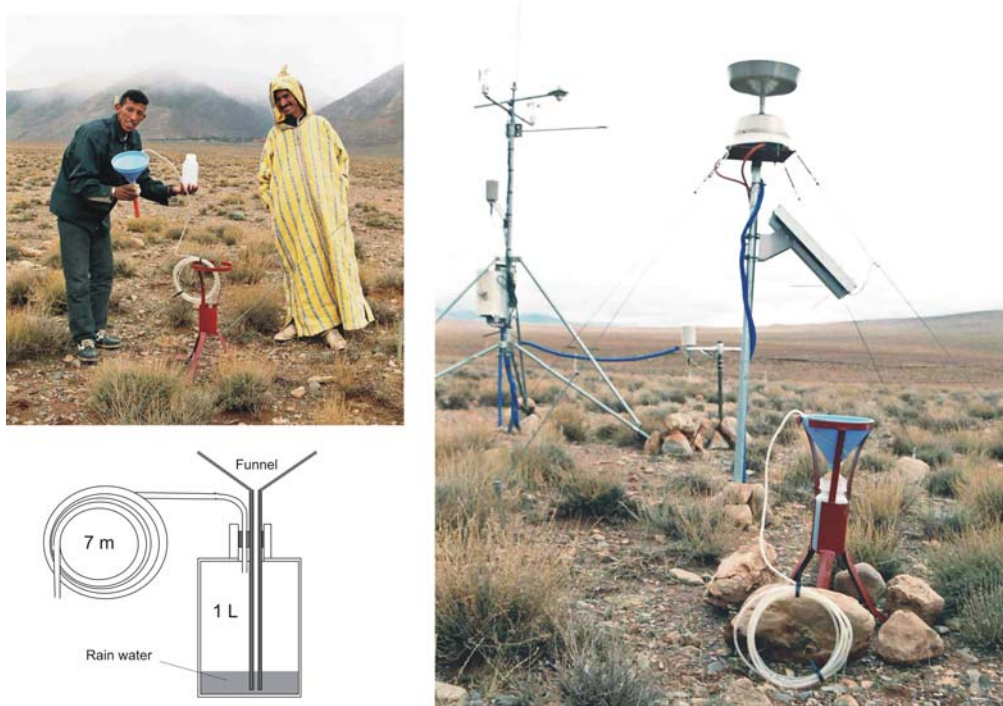
Fig. 3.4: Example of rain collector for stable isotope analyses.
