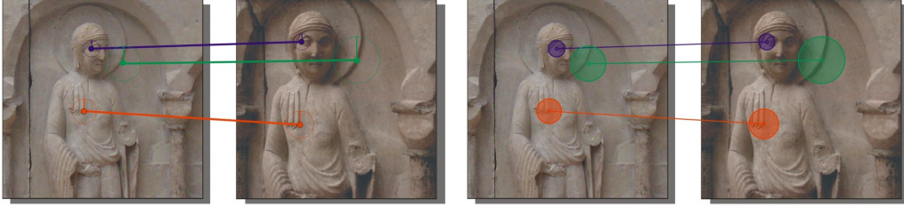
Figure 4.8: In the first registration stage, only the centres of the feature surface elements are aligned (left). The next stage aligns all available corresponding points pairs contained in the feature surface elements (right). For illustration purposes, the conforming feature matches were highlighted manually in this figure.
