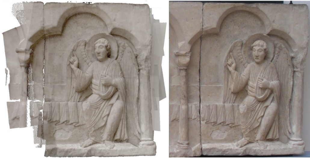
Figure 4.13: Right: Detail photograph of the rood-screen. Left: Reconstruction of the detail; 17 range images were used, no global fine registration step applied. Note that the images were taken from a slightly different viewpoint. The colour difference mainly results from using a flashlight for the photography
