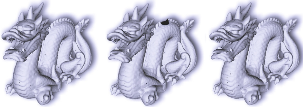
Figure 7.17: Dragon data set. From left to right: Original data set, reduced model, completed model.
