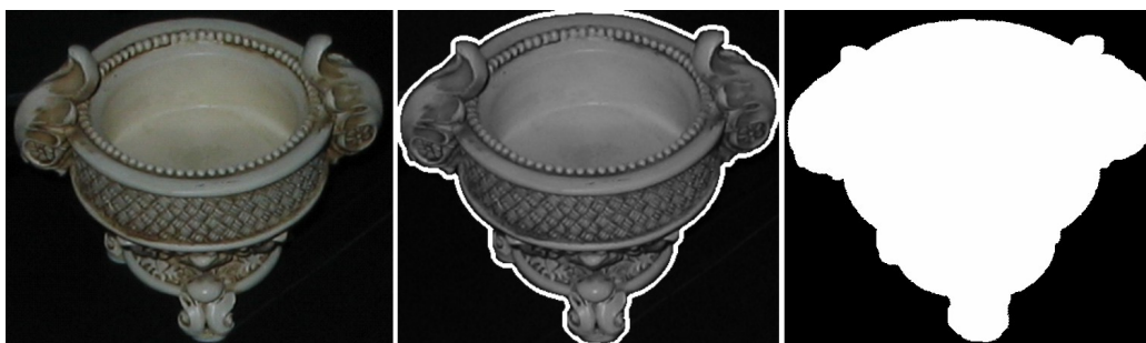
Figure 5.5: One example image \in \{I_{ii}\}_{i=1,\dots,n} (with coincident light and view direction), the extracted silhouette, and the corresponding binary inside/outside-image after thresholding.
