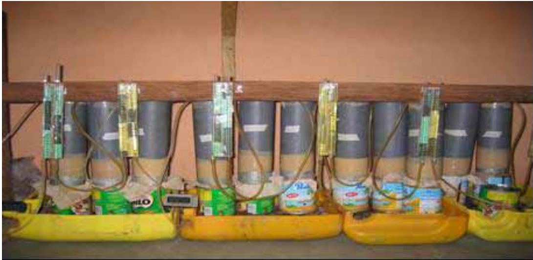
Figure 4.2 Setup of hydraulic conductivity measurements
