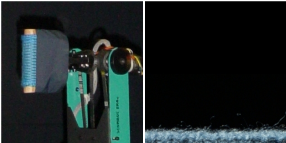
Fig. 5.18: Robot arm holding the WOOL sample and an extracted image for \theta_L = 45^\circ, \phi_L = 200^\circ
