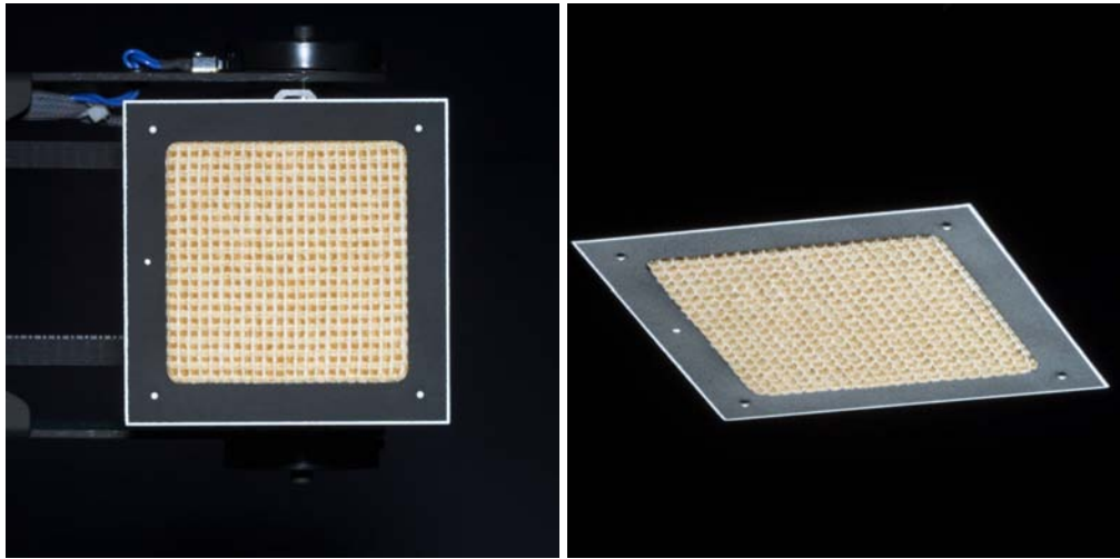
Fig. 5.6: Sample holder with the PROPOSTE sample. The left image shows the frontal view ( \theta = 0^\circ, \phi = 0^\circ ); the right image shows ( \theta = 60^\circ, \phi = 342^\circ ). White point and border markers are visible.
