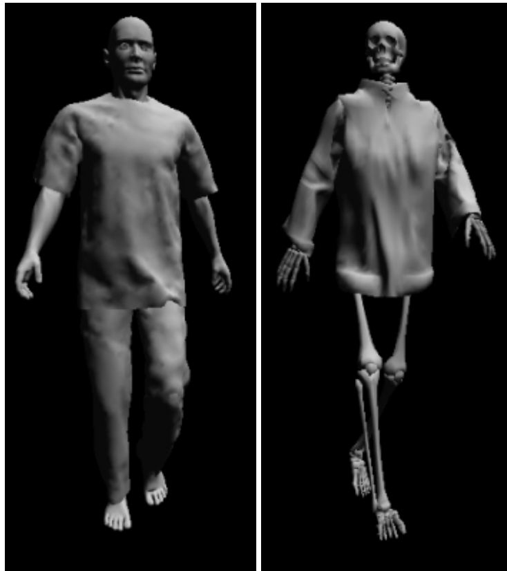
Fig. 3.4: Two models used to verify the proposed method. On the left side, the avatar model consists of three parts and has 20948 vertices. The skeleton model with another shirt on the right side consists of 12427 vertices.
