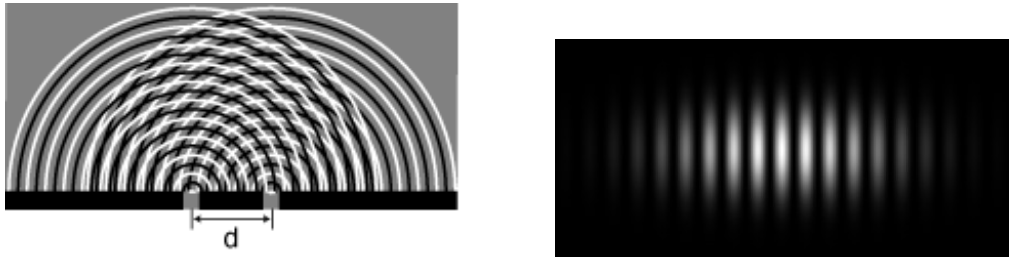
Figure 2.2: The interference pattern of light after passing through the double slit. Source: en.wikipedia.org (left figure), www.paulfriedlander.com (right figure).
