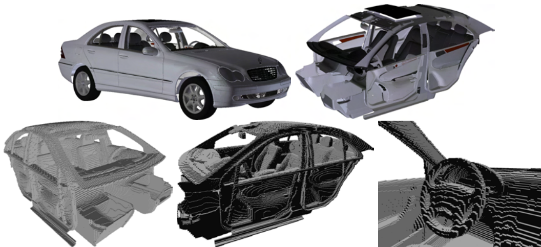
Fig. 11.12: Octree Representation of the Mercedes C class interior. Top left: complete car, right: interior. Bottom: two views of octree representation of car interior and view of the steering wheel.
