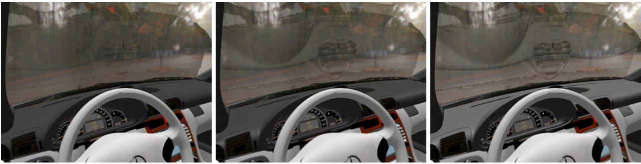
Fig. 11.17: Slight material changes drastically influence the reflections. Left: original, middle: slight specular factor added, right: slightly increased diffuse and specular reflection properties. Such cases should be detected using Virtual Prototyping.
