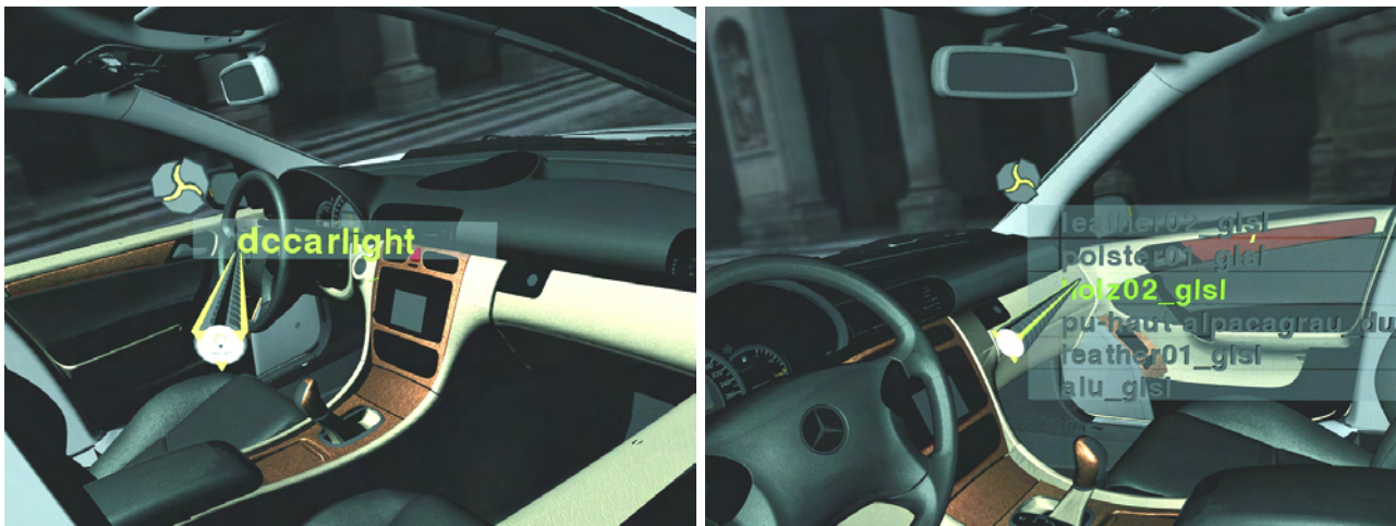
Fig. 14.1: Light and material selection in the RealReflect system. (image courtesy of IC:IDO GmbH)
