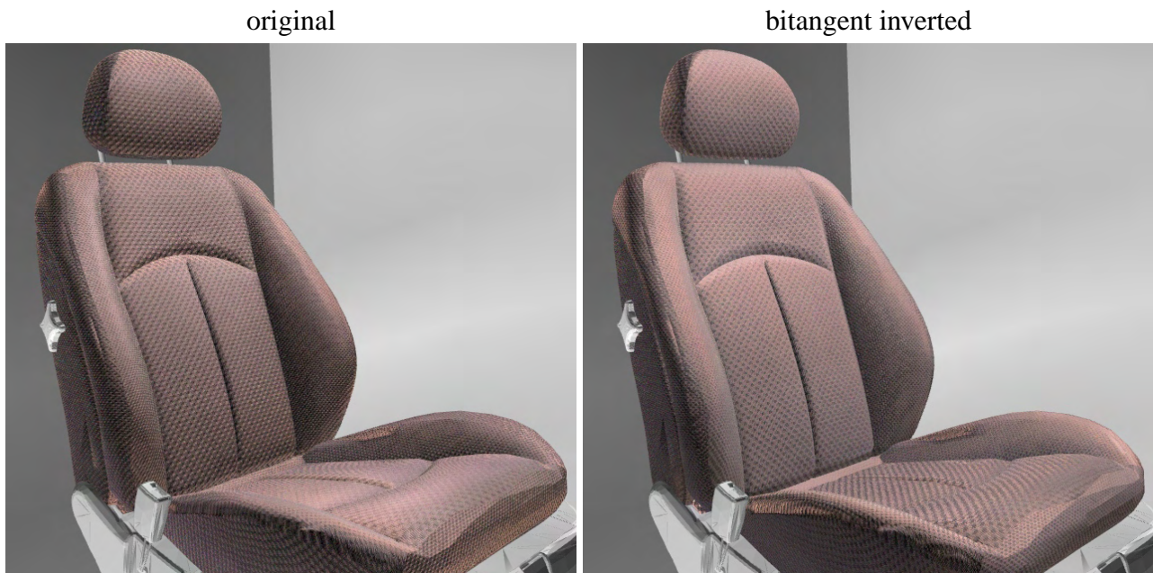
Fig. 14.4: Change of appearance due to inverted bitangent in local coordinate system. Phong BRDFs typically used in VR applications lack such anisotropic behavior.
