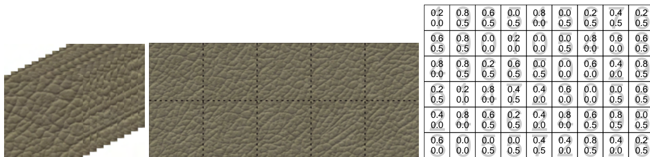
Fig. 9.8: Data for rendering tiled BTFs. Ten tiles (left) arranged in a single texture T_p (center) with (c_{T_p}, r_{T_p}) = (5, 2) , right: tile matrix T_i with (c_{T_i}, r_{T_i}) = (9, 6) storing offsets for respective tiles in T_p (tile numbers are printed in large, gray numbers).
