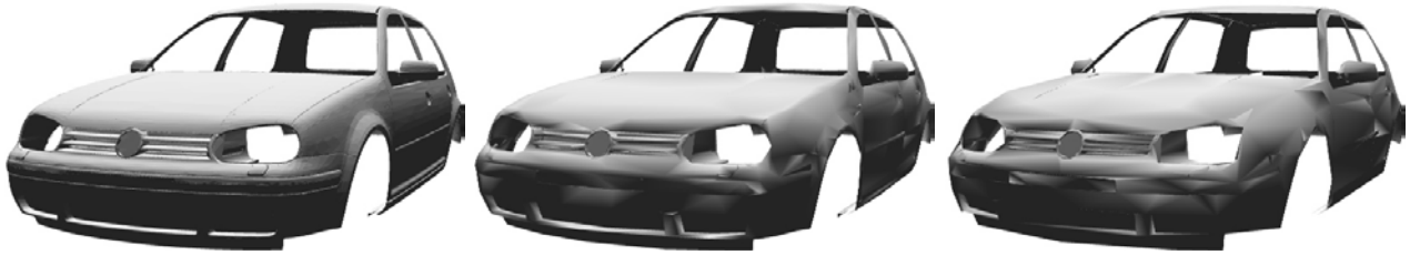
Fig. 5.8: Static LODs of a VW Golf car body. Left: original (43k vertices), center: 3 mm geometric error (7k vertices), right: 1 cm (6k vertices).
