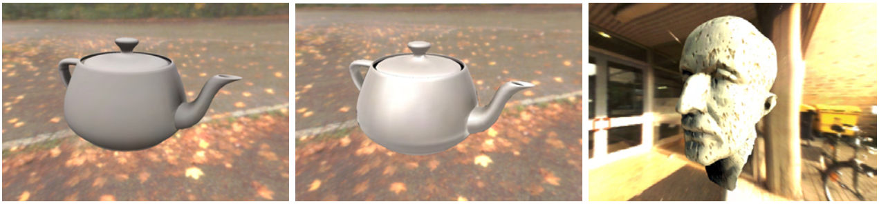
Fig. 8.4: Extending PRT to more general materials. Left: diffuse BRDF, center: Phong BRDF, right: plasterboard BTF.
