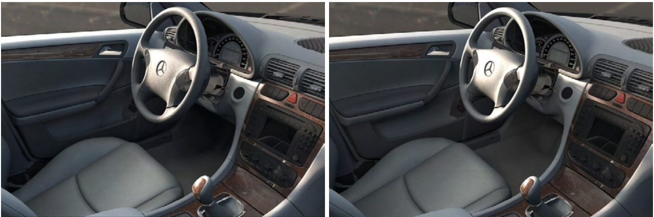
Fig. 13.12: Changes in rendered images due to approximated indirect light. Left: direct lighting only, right: an additional area light source simulating indirect light in the interior.
