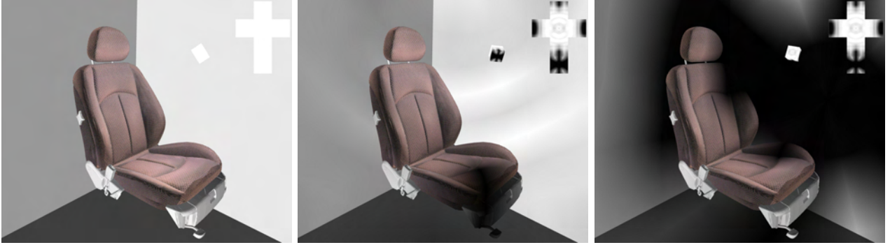
Fig. 9.5: Rendering with point light sources emitting radiance equally into all directions (left) or according to a goniometric diagram (other). Light sources are rendered as textured cubes, their goniometric diagrams are shown as cube-map crosses.
