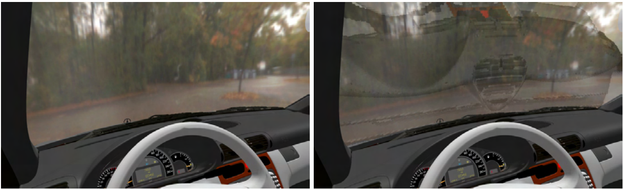
Fig. 11.10: Windshield of a car without (left) and with (right) interactively rendered reflections.
