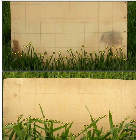
Figure 3.10: Digitalisation of the vegetation profiles, using a point distance of 2cm. Exemplarily shown for 04/12/2006 (tillering) and 06/07/2006 (heading).
