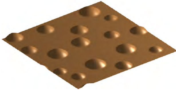
Figure 1.6: A typical configuration of well-defined equilibrium droplets connected by a uniform precursor layer on a periodic domain.
