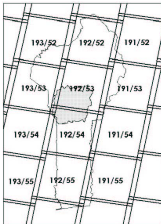
Fig. 2.3: Coverage of Benin by Landsat imagery. The coverage of the HVO area demands a mosaic of Landsat scenes 192/53 and 192/54. (from JUDEX 2003).
