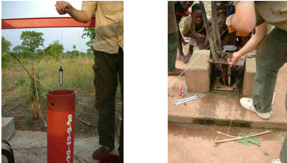
Fig. 2.5: Installation of the automatic data loggers in observation wells (photo a) and footpumps (photo b) with authorisation by the villagers and in cooperation with the technical staff of the beninese water ministry.
