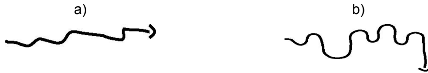
Fig. 3.12: a) The water course is controlled by fractures (“en baionette”). b) Sinuosity depends on morphological features and not on fractures (from CEFIGRE 1990).
