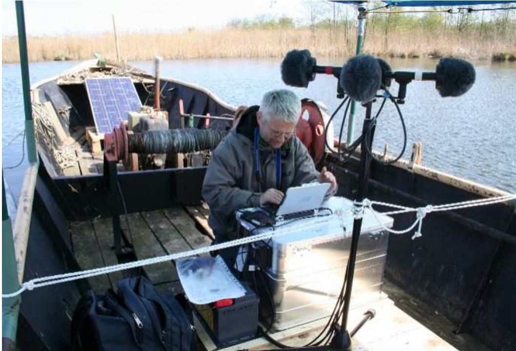
Figure 5.1: An autonomous recording station powered by solar panels is dispatched on a boat.
