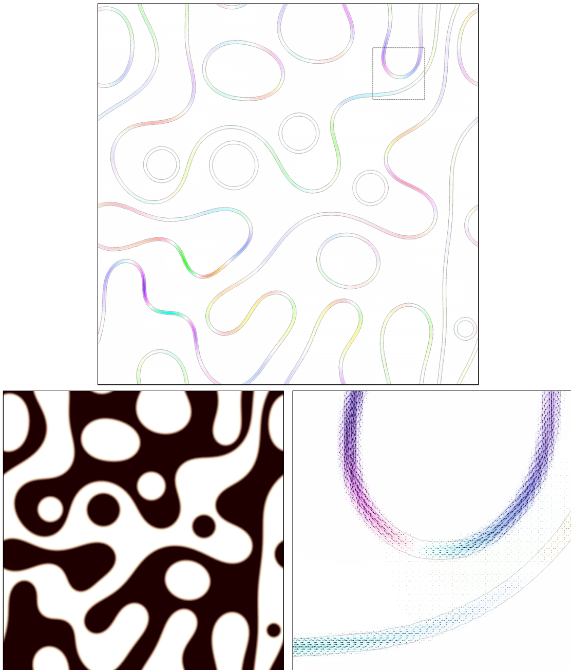
Figure 5.13: The upper picture shows the flux in a variable quench simulation: the hue shows the direction and the saturation shows the magnitude of the flux (see circle on the right). Clearly visible is that the flux goes along the interfaces (grey lines), as expected for an approximation of surface diffusion. The lower pictures show \phi (left) and a detail of the upper picture (right).
