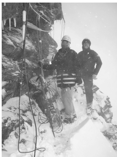
Fig. 24: Test measurement of frozen rock surface resistivity values at the NE transect (August 15, 2005).
