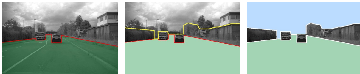
Figure 7.5: Estimation of the Free Space Band. The free space (middle image, green) is the instantaneous space free of any obstacles. By using an object height segmentation, the free space band is derived (right image). This free space band contains all important objects for autonomous decision making.
