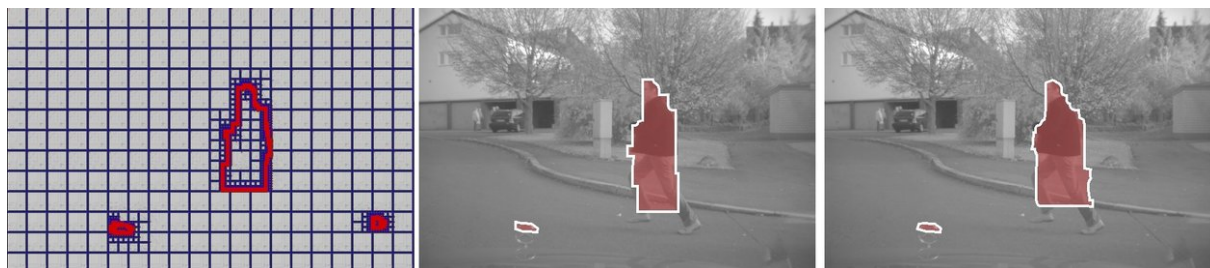
Figure D.6: Segmentation using the multi-resolution method in comparison to the full graph-cut method. The left images show the multi-resolution graph and the corresponding segmentation overlay. The right image shows the results using full graph-cut, yielding similar results.
