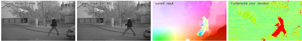
Figure 4.21: Optical flow for a scene with a running person and a moving camera, installed in a vehicle. The distance to the epipolar rays encodes independently moving objects.
