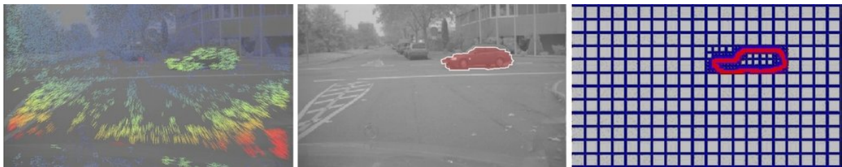
Figure D.1: The images show the flow field of image features in a traffic scene and a segmented moving object. The image on the right shows the multi-resolution graph structure obtained using the approach in this paper for real-time segmentation.
