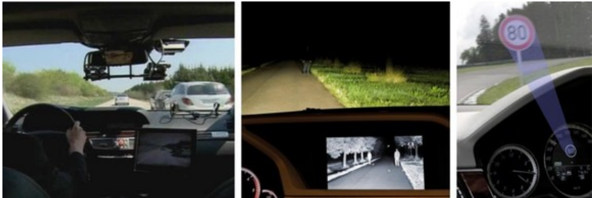
Figure 1.1: The left image illustrates the camera setup in the demonstrator car. The middle image shows the Night Vision System [17] and the right image the Speed Limit Recognition, two computer vision based assistance applications in the new Daimler E class (W212 model).
