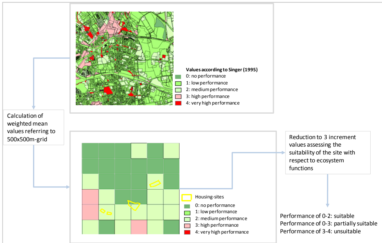
Figure 13 Grid-based calculation of the regulative performance and the biotope quality of cadastral land use data (author's draft, Data-source: Cadastral Land Use Data (ALK), Office of Geoinformation, Measurement and Cadastre, City of Essen/Amt für Geoinformation, Vermessung und Kataster der Stadt Essen (2007))
