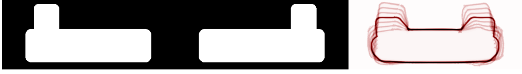
Figure 5.5: Average and variation (right) for two shapes with pins at different positions (left). The pins are not interpreted as shifted versions of each other.
