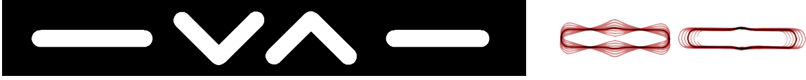
Figure 5.1: The two dominant modes (right) for four different shapes (left) demonstrate that the principal component analysis properly captures strong geometric nonlinearities.
