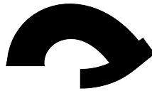
Figure 7.9: Local equilibrium deformation for the mechanical problem in Figure 7.7 which reverses the orientation of the crossbeam and cannot be reached starting from the configuration in Figure 7.7, left.
