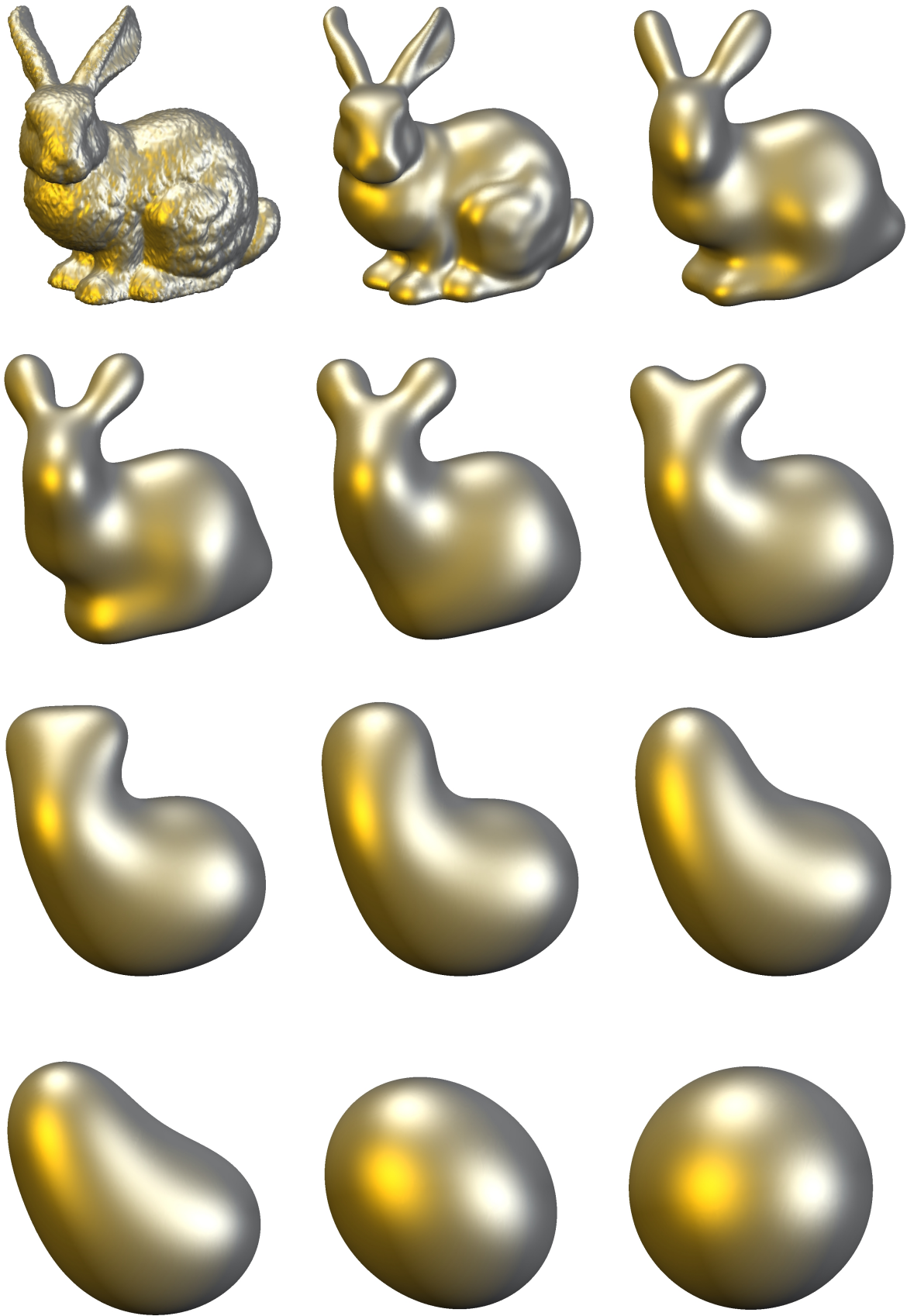
Figure 4.14: Evolution of the Stanford bunny [2] towards the sphere. The grid consists of 40648 nodes and 81292 triangles. The time step size equals the spacial grid size. \tilde{\tau} = \tau^2 .
