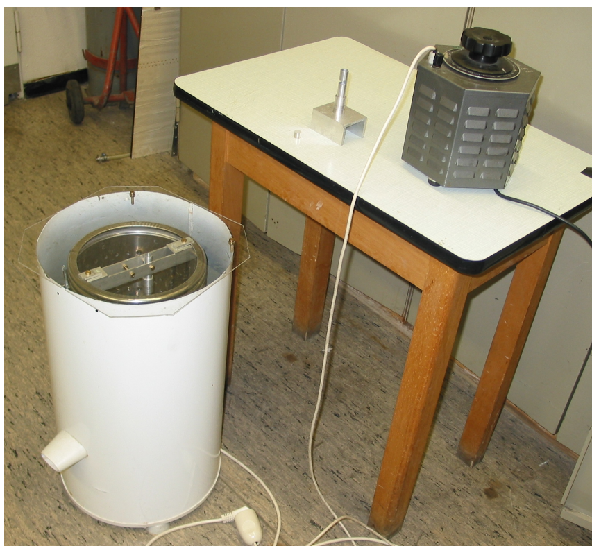
Figure 3.4: Experimental setup for sedimentation process of the MNPs. It consists of a centrifuge, a transformer, a cylindrical tool, and a sample vessel.
