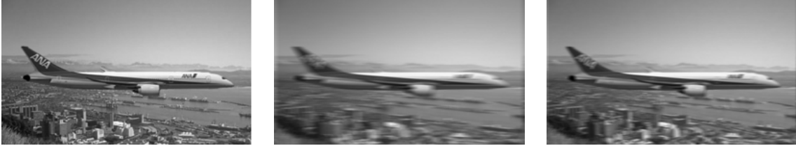
Figure 4.3: Most basic motion deblurring: Original image f (left), an artificial input image generated by (4.5) (middle) and reconstruction obtained by minimizing the energy given in (4.6) (right).
