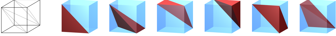
Figure 3.2. Subdivision of a cube into 6 tetrahedra. The diagonals on the left and right, top and bottom, and front and back faces are pairwise consistent with the neighboring cube, hence the resulting tetrahedral mesh \mathcal{G}^{\boxtimes} is admissible in the usual sense (see e. g. [55]), in particular there are no hanging nodes. The angles of the regular tetrahedra lie in \arccos\{0, 1/2, 1/\sqrt{3}, 1/\sqrt{2}, \sqrt{2}/\sqrt{3}\} \approx \{90^\circ, 60^\circ, 54.74^\circ, 45^\circ, 35.26^\circ\} .
