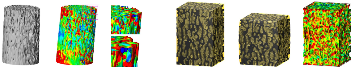
Shearing simulation for a cylindrical specimen of porcine trabecular bone. Zooms to one corner of the specimen are shown on the right. All deformations are scaled for better visualization.
