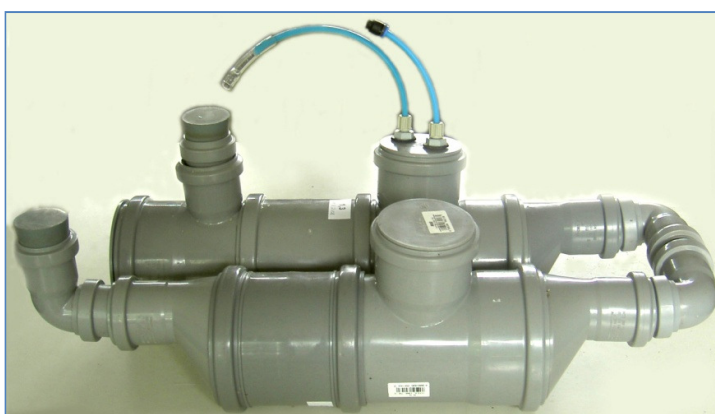
Figure 2.3 | Constructed 2-chamber septic tank model.
