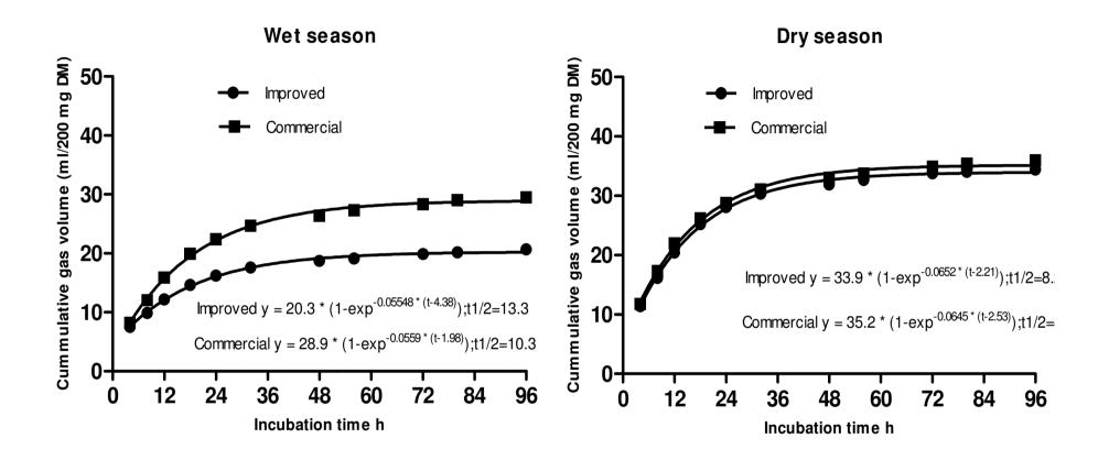
Fig. 1: In vitro gas production profiles of the cowpea haulms at wet and dry seasons. Gas production profiles have been fitted to curves using the equation ( $y = B^{(1-\exp^{-c^{*}[t-lag]})}$ ) with time to half maximal gas production ( $t^{1}/_{2}$ ) expressed in hours. Standard errors for maximal gas production and rate of gas production for wet season were 0.18, 0.0031; 0.29, 0.0032; for dry season, 0.23, 0.0029; 0.31, 0.0036 for improved and commercial haulms, respectively.
