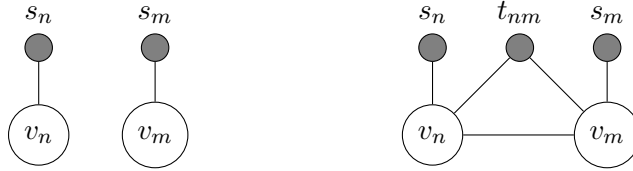
FIGURE 4.7: Graphical representations for the minimal matching problem depicted in Figure 4.5. Left: Model for descriptor-based matching, assuming independence between the variables, and using only descriptor dissimilarities s_n, s_m as observations. Right: Proposed model, including the pairwise dependency (v_n, v_m) \in \mathcal{V} \times \mathcal{V} between the variables, and observing a geometric inconsistency t_{nm} .
