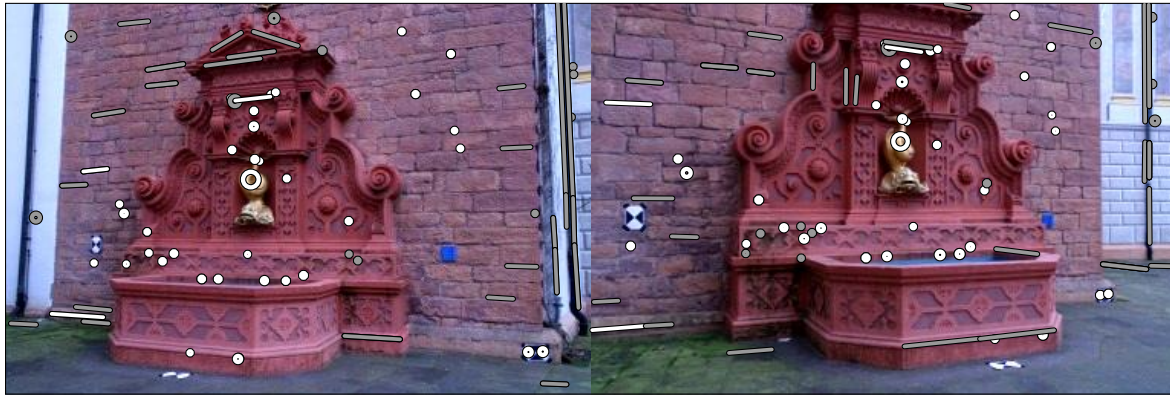
FIGURE 5.2: Example image pair from the FOUNTAIN-P11 dataset, showing a set of feature correspondences that have been automatically annotated using the procedure described in Section 5.3. As in Figure 5.1, white features are classified as correct, and grey features are classified as outliers.
