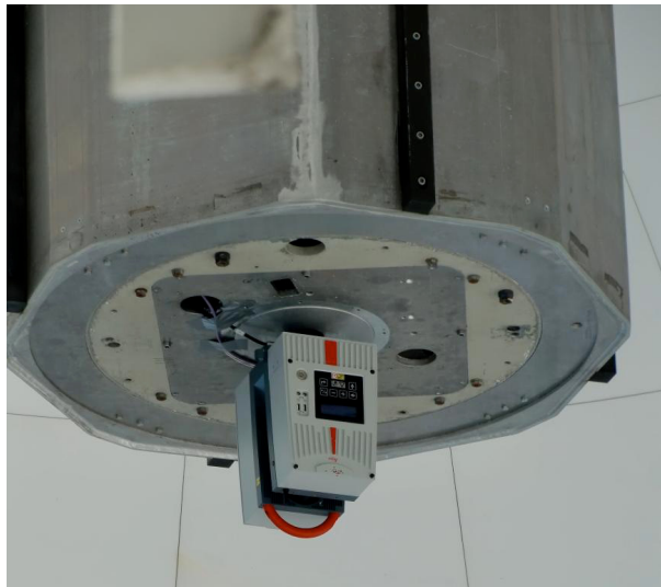
Figure 3: Upside-down observing station of the laser scanner inside the subreflector at an elevation angle of 90° of the main reflector.
