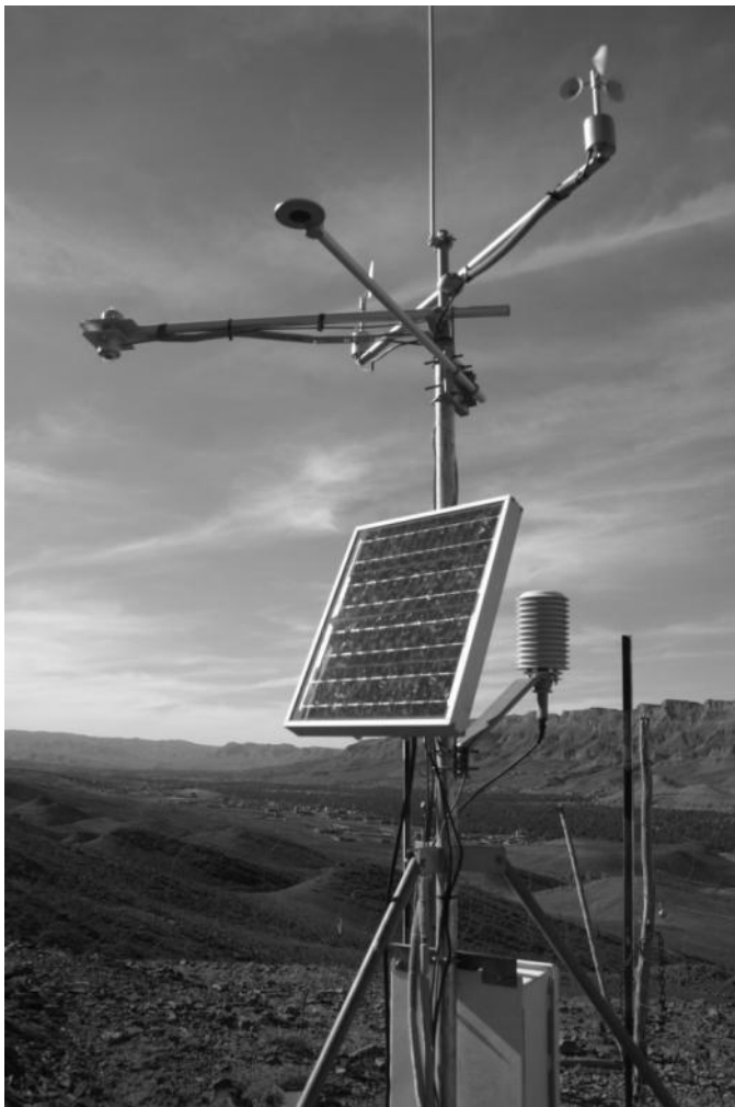
Figure 26 Automated Climate station ARG with of wind, temperature and radiation sensors.
