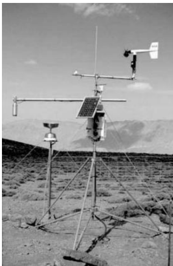
Figure 4 Automated Climate station as operated by IMPETUS (TZT Station ~3000m asl.)
