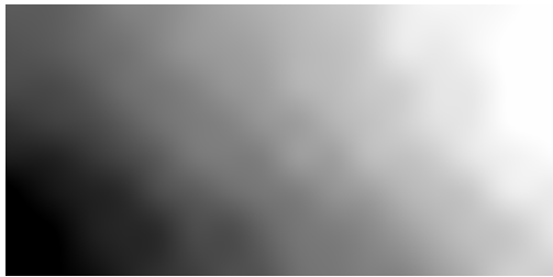
d: Illumination correction; the levels in this image vary by \sim 7\% (300 ADU).
