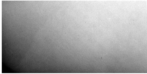
b: Flatfield; the counts drop by \sim 25\% from the upper right to the lower left corner (due to vignetting of the telescope optics).
