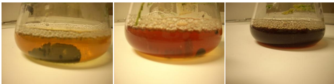
Figure 4.2.2-2: 300 ml culture flasks containing cyanobacterial cultures of F. ambigua in BG-11 after 3-4 weeks (left), 6 weeks (middle) and 2 months (right).
