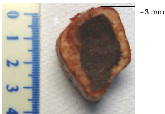
Figure 8: Bovine rib segment with cortical thickness of about 3 mm.
