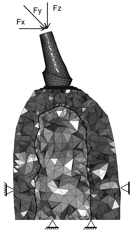
Figure 12: Boundary conditions of the numerical models.
