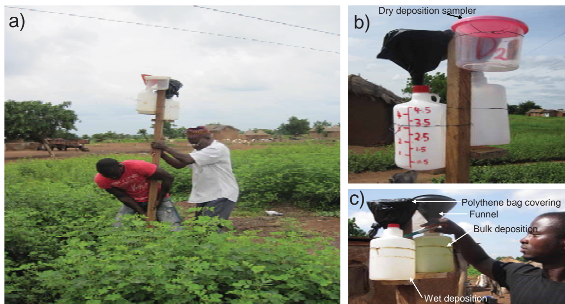
Figure 5.2 Wet, dry and bulk atmospheric deposition samplers as mounted in the field. a) Entire apparatus as mounted in the field. b) Dry deposition sampler. a) Wet and bulk deposition samplers showing observed biological activity in bulk depositions but no such activity in wet-only depositions.
