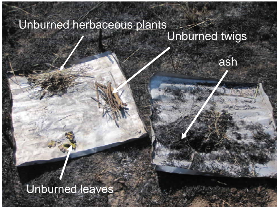
Figure 4.4 Field pre-processing of burned vegetation into unburned parts (unburned herbaceous plants, unburned twigs and unburned leaves) and ash component
