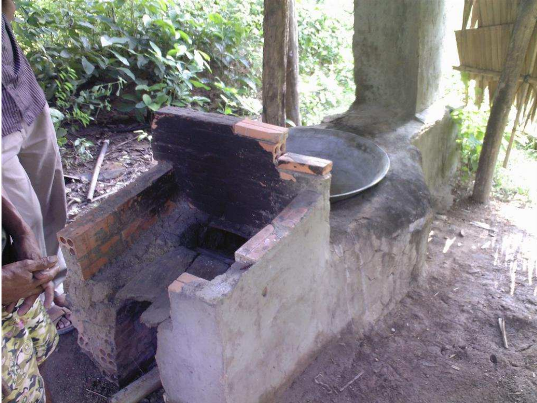
Figure 4.5 Custom-made palm sugar cookstove based on NGO-developed designs, Kampong Speu province
