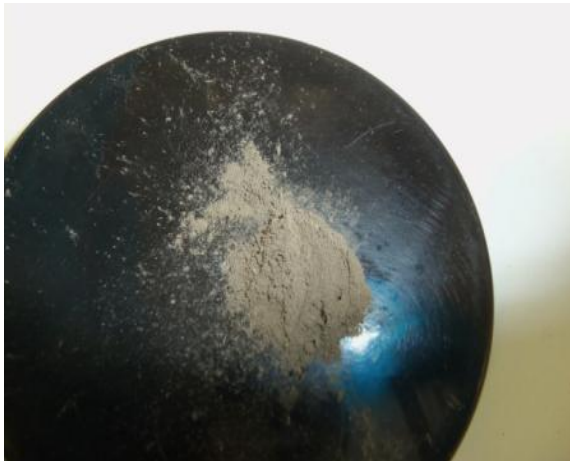
Fig. II-28: Struvite precipitate after drying at 50°C
