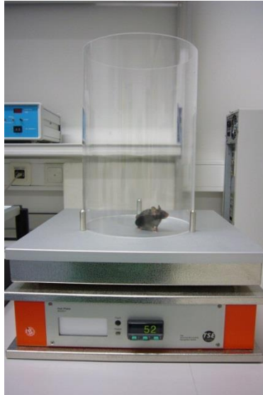
Figure 5: Hot plate test device. The animal was placed on a heated surface (52°C). Next, the latency to the first pain reaction (shaking of the hind-paw) was measured
