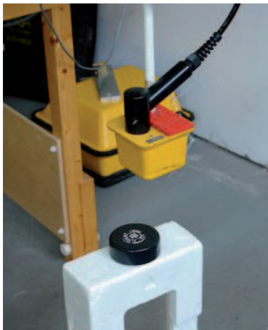
Figure 2.10 – View of GPR Transmitter/Receiver Head.
