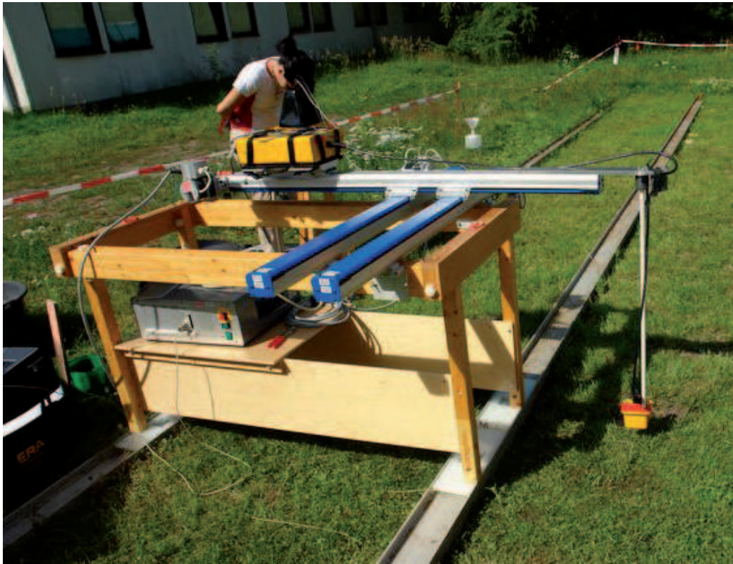
Figure 2.11 – Test field and SPRScan Radar in the LIAG (Hannover).
