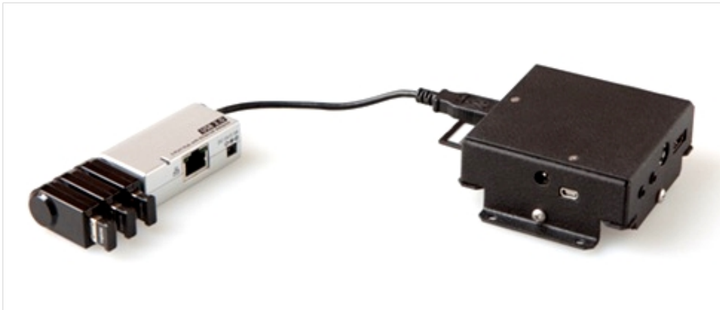
Figure 4.1: Bluetooth Scanner developed at Fraunhofer IAIS.
