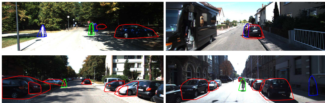
Figure 5.8: Detection results of the mixture of bag-of-words for cars (red), pedestrian (blue), and cyclists (green). We show the convex hulls of the projected laser range points.
