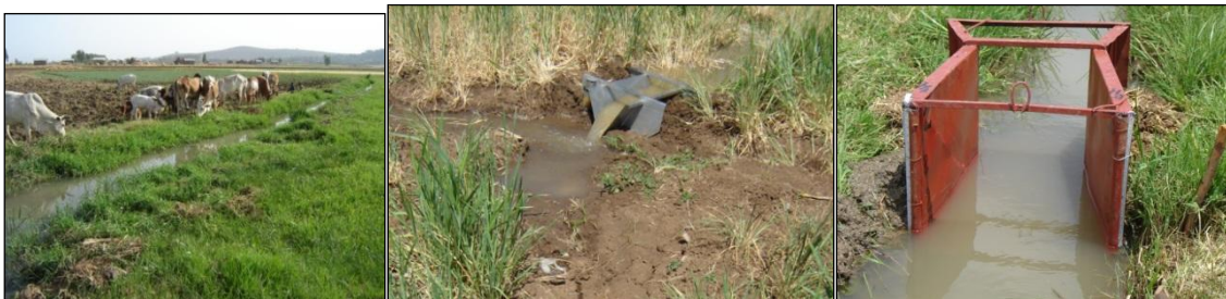
Figure 4-5 Grass production along main canal (left), Replogle-Bos-Clemmens flume (center) and cutthroat flume (right)
